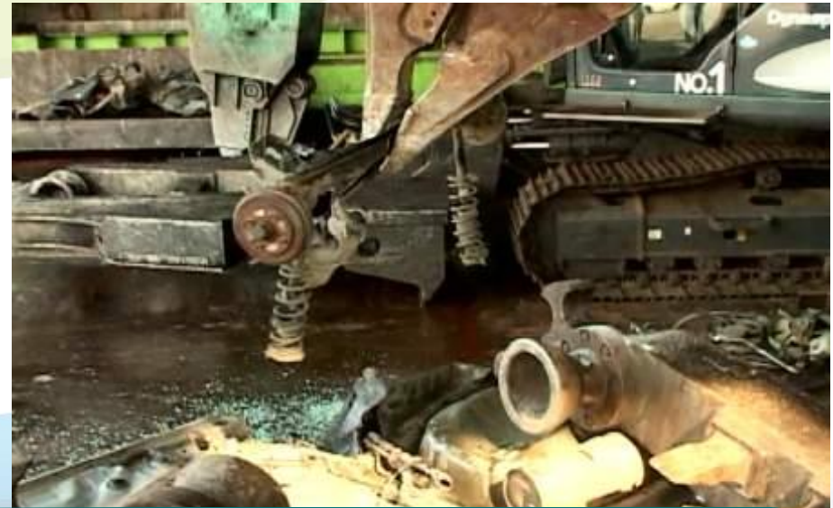
Rear suspension removed
