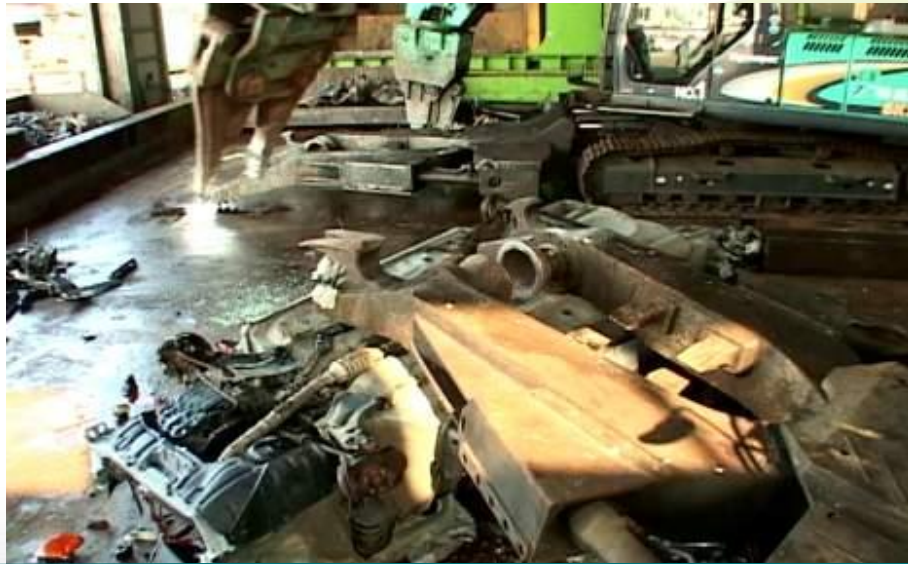
Car body secured in clamp arm
