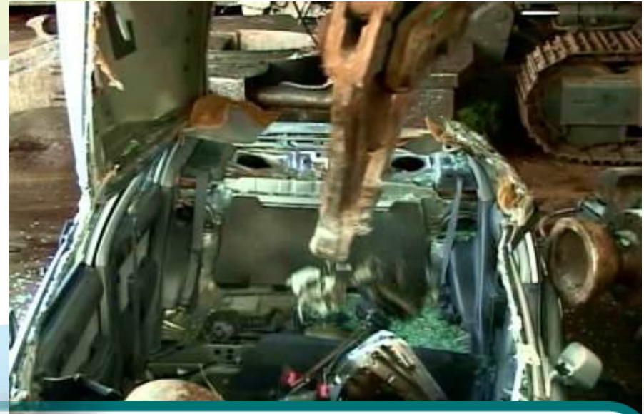
Electric wire and harness under seats pulled off
