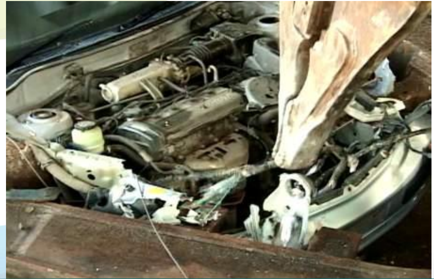
Electric wire and harness pulled out from the front
