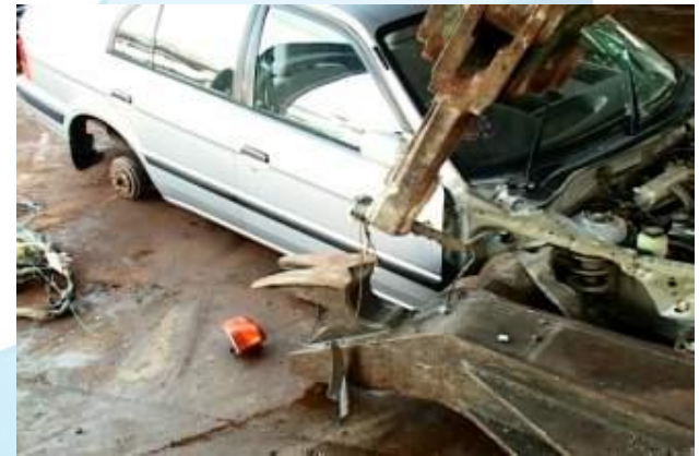
Electric wire and harness removed by fork pointed tooth
