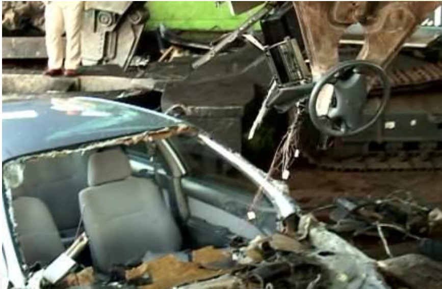
Steering wheel and dashboard panel removed
