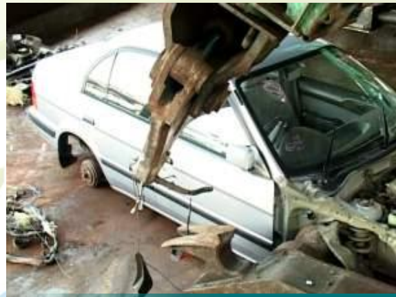
Electric wire and harness removed by fork pointed tooth
