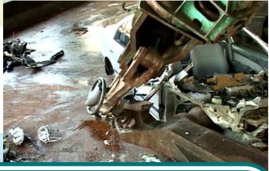
Panel separated by fork pointed tooth
